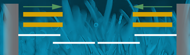
VG 17 (centre opening) + 4 sliding panels, 2-track
