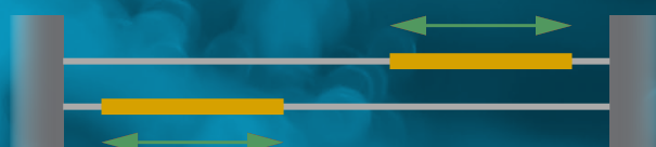
2-track the number of sliding panels can be selected
