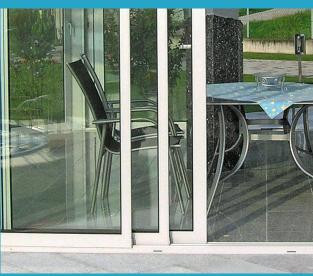
All elements in this system are free sliding, with the element running inside equipped with a multiple seal and window handles, the outer with a recessed reversible handle. The use of high-quality double rollers guarantees permanently smooth sliding even at element weights of up to 221 lbs.
